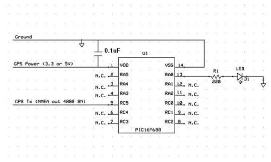
**Figure 2 The Schematic**
