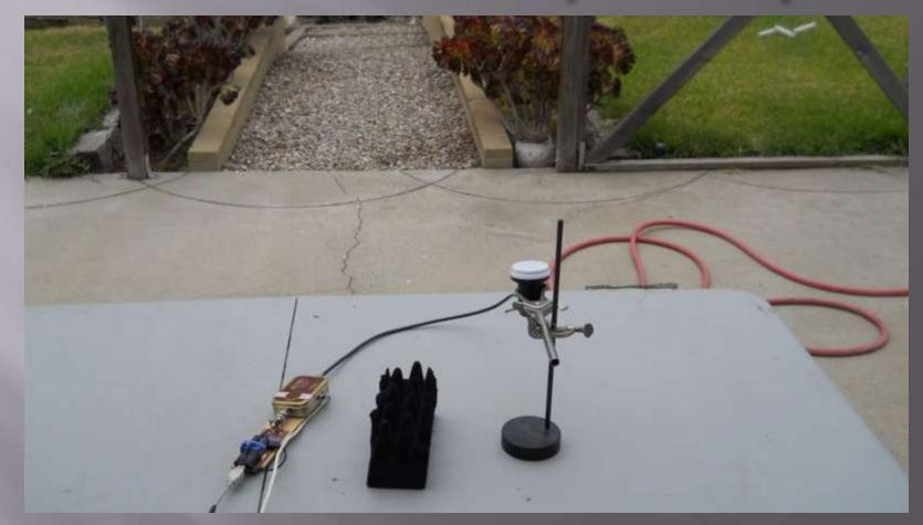
Rein takes advantage of the excellent front-to-back ratio of the Ku band feedhorn to reject ground noise. Plus it is pointed as far away from the ground as practically possible.
