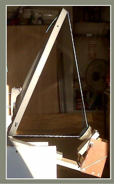
WIGHZ developed a very useful method of finding the focal point with a string.
