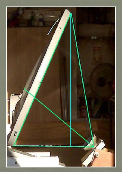
Bisect the offset reflector vertical illumination angle and that's the spot to point at, not the center of the reflector.
