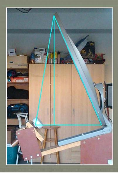
When making measurements on your dish, measure to the edges of the reflective surface. rather than the outside lip of the sheet metal. This will yield better agreement with calculated values.
