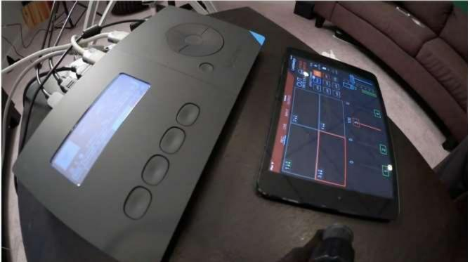
Its onboard WiFi connects without wires to the JetPak hot spot mentioned above. The Cerevo Livewedge is controlled either by the four buttons on the hardware, or through a digital interface, in this case, the Asus tablet to switch cameras and to insert graphics (Callsign ID) during the meeting.
