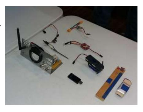
model telemetry. The airborne X-Bee transmitter is the red thing. The sensors are for air speed (pitot tube) and motor current. He talked about the use of folded steel (hardware store gutter flashing) instead of a project box. It makes for a convenient and very cheap chassis.
