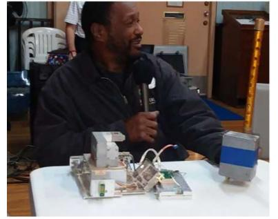
(The caption here is from Dave Laag.) From left to right: Items brought to the meeting for giveaway include Western Electric LO assembly and aircraft X-band weather radar down-converters. Robert Carter is holding a low power 10.368 GHz omni-directional beacon built he built. According to Robert, the antenna seems to have some-what equal vertical and horizontal components.
