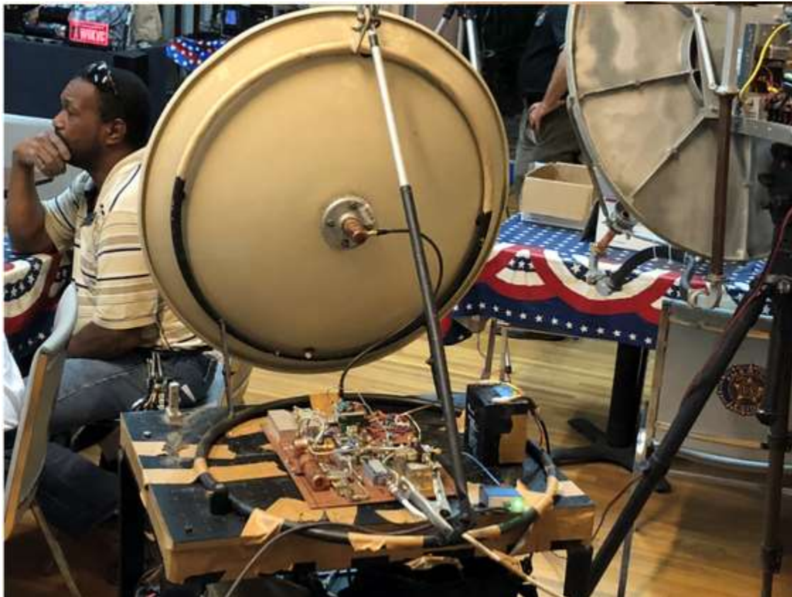
Bob Carter KM6RXN and his first 10 GHz rig. Note very light, yet very rigid method of elevation adjustment.
