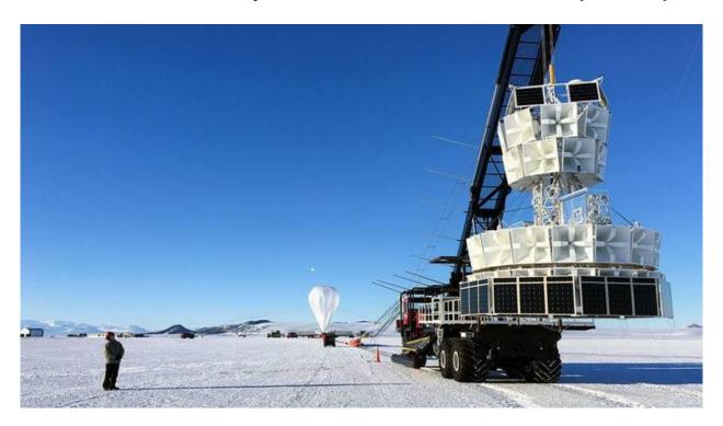
Recognize the ridged horn construction? Notice that the E field response is both polarization orientations. It is for the detection of Cherenkov radiation in the UHF emitted by ice from neutrinos entering the other side of the earth. This uses the earth as a neutrino-pass filter.
