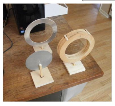
They are rings of just the right inner and outer radii so that the diffraction is just right for constructive interference at a single point. They are Fresnel lenses. The metal ones reflect away energy whereas the wood one which is of just the right thickness will delay by ½ wavelength so that this opaque ring actually contributes also. The
