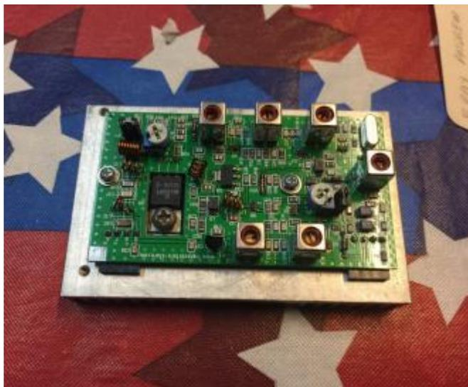
meter to 2 meter transverter that was \$55 and puts out 6 watts. Models for 6 m. and 70 cm. are also available, fully tested. (See picture.)
