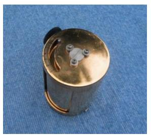
Bill Locke N6WL told us that it is the temperature control cavity for a Klystron. The screw on the side adjusts the frequency of the Klystron. Adjustment on the back adjusts the temperature.
