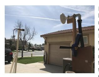
I've collected several feed horns from Ku band systems and used them for my X Band rigs. These horns were designed for 12 GHz TV systems, but I'm using them at 10 GHz. I assumed they had wider beam widths at 10.368 GHz, but how much wider? Does it matter? I decided to test my offset feed horn collection to find out what their actual patterns were at 10.368 GHz. Some of these horns have been
