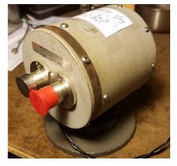
← This is the PRD 670 thermopile AC/DC transfer standard. AC or DC input equals a known DC output.
