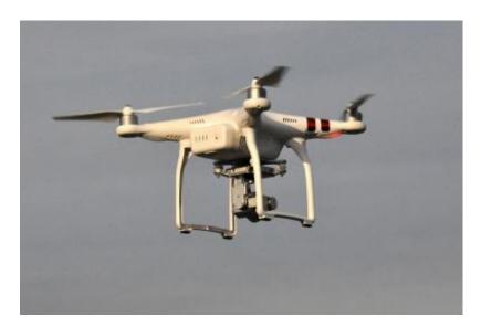
One manufacturer sold about a million "quad copters" in the U.S. alone in 2015. What does this have to do with microwaves? They use the 5.7 GHz band to send high resolution video from the vehicle to the ground video display or even a head mounted display. The RC-to-aircraft control link is the 2.4 GHz Wi-Fi band.
