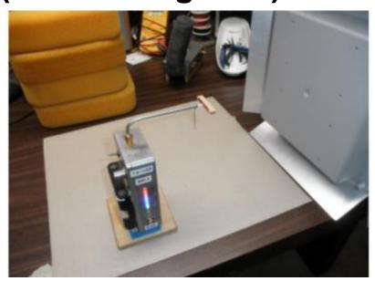
The antenna on this field strength meter is about the correct size for the 2.4GHz signal it is bathed in.
