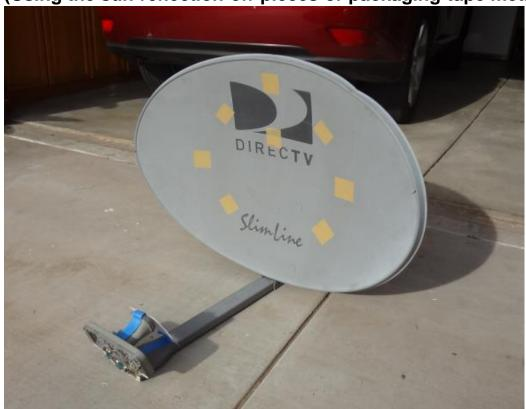
This is a DirecTV "Slimline" reflector that is normally fitted with 4 LNBs. Note (below) that I found the best focus point is below the feed by about 2
