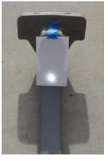
inches. Also note I only put a tape-reflevtor in the center part of the reflector to avoid confusion from the sides. I intend to use a circular offset feed. I'm hoping for about 33 dB gain.
