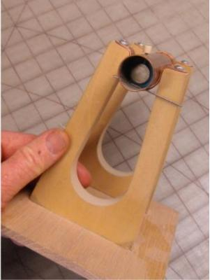
Hint: that's a tungsten rod across the bottom and a tungsten disk in the tube. Through the BNC on the back, it's powered by 3,000 volts DC. And yes, it is a microwave device.
