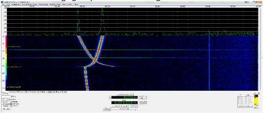
Below, both LNBs were pointed at the Santiago X-band beacon at 10368.330 MHz (– FCD + IF tuning to 618.500 MHz). Left and right LNBs were interrupted on purpose (by power cycling sequentially for 10 seconds to show which LNB was which.) Followed by power interruption to both to show background noise.
