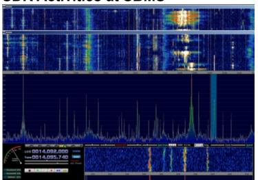
Here Rein captured some action with his WSPR mode software and an \$18 dongle. (20 meter band: 14.0956 MHz)
