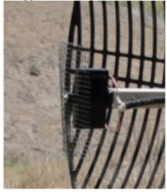
antenna for the 1.2GHz. Like Gary's antenna outside our meeting place, the 2.4 GHz is for transmitting to Santiago and 1.2GHz is for receiving from Santiago.
