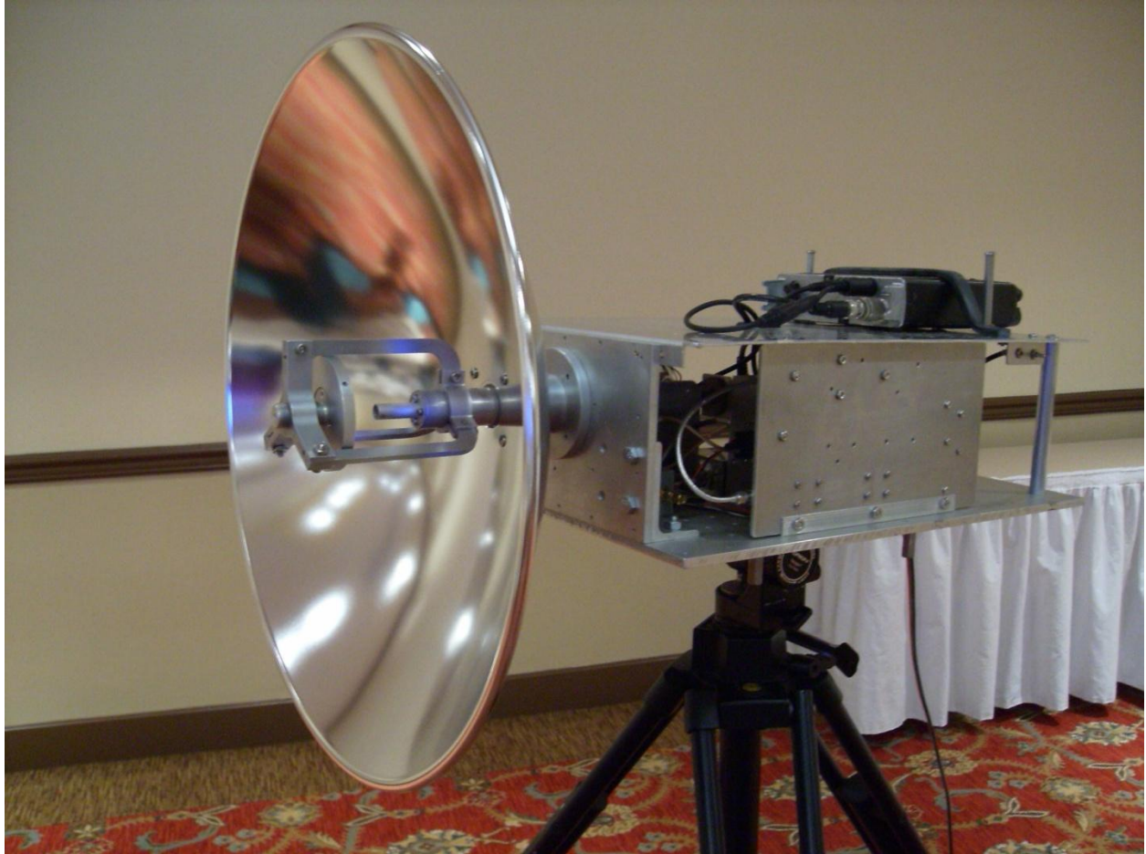
A 47 GHz rig at MUD 2012 was of nice design with an FT817 IF radio sitting on top.
