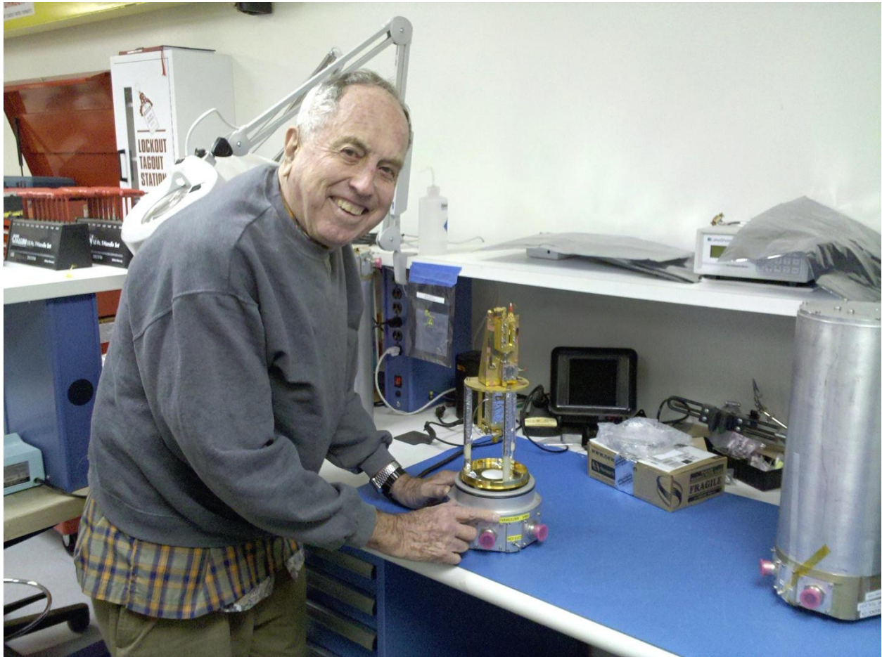
Paul Lieb (KH6HME SK) checking out the 600GHz LNA used at the sub millimeter antennas, Smithsonian Astrophysical Observatory, Mauna Kea, (Big Island) Hawaii. Notice static strap on Paul's left wrist, the LNA is valued at $300K.
