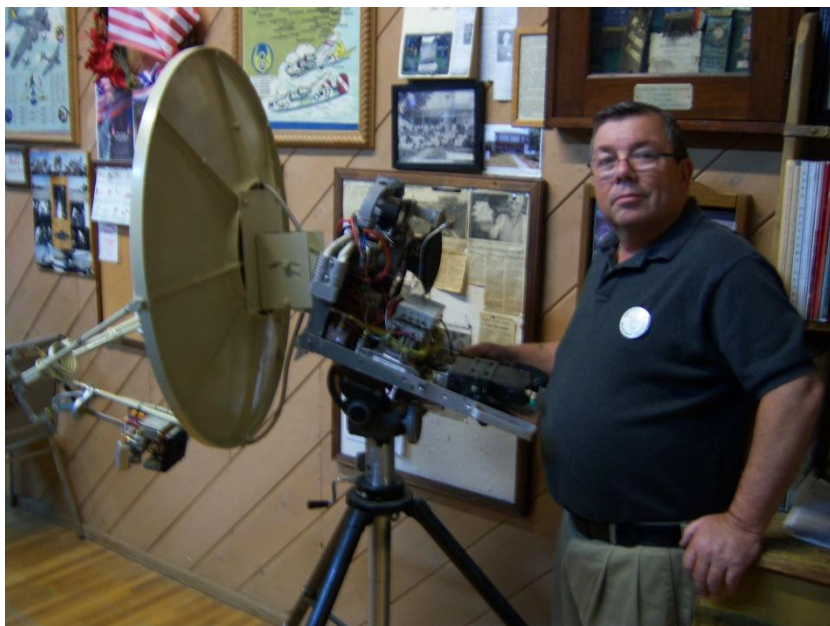
Pat, N6RMJ with his dual band 10 and 24 GHz rig. The 24 GHz section is seen on the feed arm while the IF radio and 10 GHz section is just above the tripod head. Nice modifications to the previous single band rigs.
