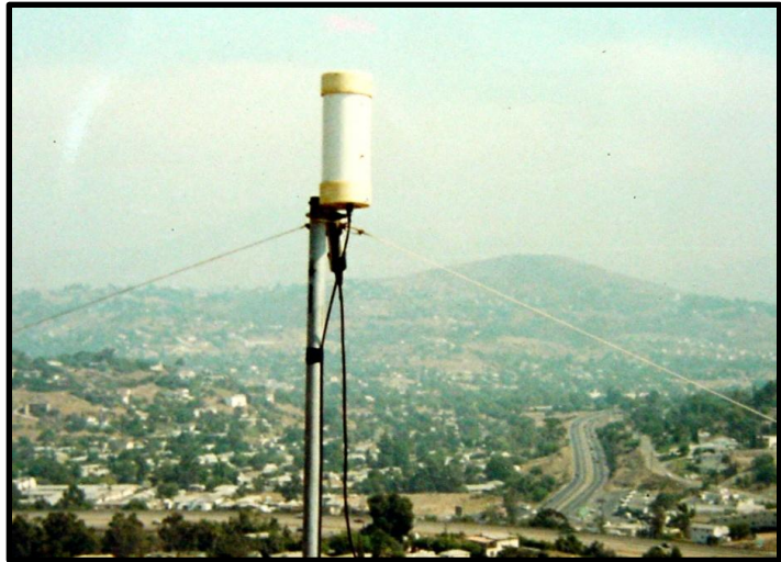
Figure 8. The N6IZW/R beacon mounted on the roof of W6BLK's home. It consisted of a Gunn diode into a slotted line antenna. The Beacon was later moved to Palomar. Photo courtesy of N6IZW
