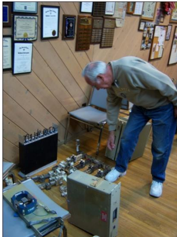
Larry, K6HLH checks out some of the waveguide assemblies and klystron amplifier/ power supply units.
