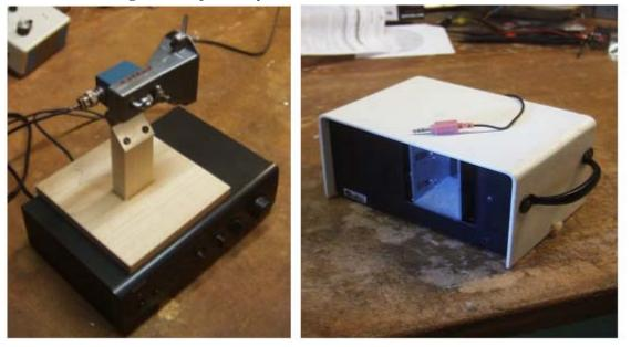
transmitter assembly. It is a motion sensor modified with the mini-phone cable and two small resistors attached to the Gunn diode. My own microwav e interests are primarily with the
