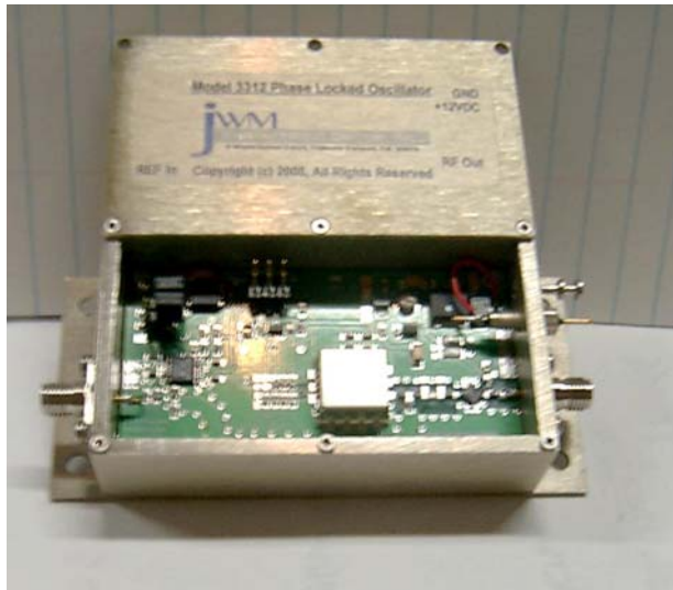
JWM Engineering prototype 3.4 GHz LO for the SBMS 3.4 GHz transverter project. It has good phase noise properties for the project unit.
