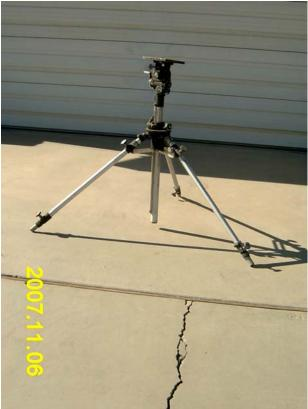
The Quickset Majestic is a nice mount that has about all the features you would like on a tripod. One thing that Chip, N6CA likes to do is add an extension to the leg to vertical member where the legs can extend really wide and give the tripod the maximum stance to keep the wind from overturning your antenna and gear.
