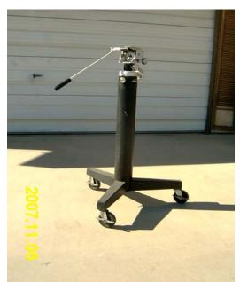
The Quick Set Sampson mount is great where you have a level floor to roll on. It has the azimuth and elevation adjustments. The rig does need a 1/4 –20 screw mount to bolt on to the platform of the head. There is a version of the Sampson that does have legs.
