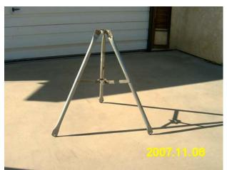
The roof mount tripod lacks adjustment for uneven ground. You could take out the crimped feet and use coaxial conduit to make the legs adjust.
