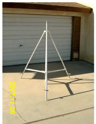
Sometimes you find a large tripod that is five feet tall. In this case there are leveling extensions on each leg to adjust for uneven ground. But it is too tall for the average amateur to reach his equipment mounted on top.
