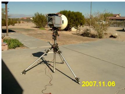
The Majestic also has a vertical adjustment to allow the antenna to move up and down. Sometimes a couple of inches to clear that fence is nice to have. Bill WA6QYR
