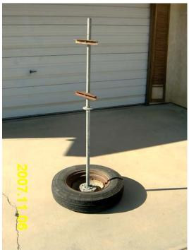
You can use a vehicle wheel/ tire to place a pole vertical and brackets to hold the dish. This you can roll to the site, but needs a level site to park on. The two pipe floor mounts make a rotator and a smaller pipe holds the two sections of pipe together in the vertical.
