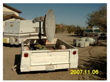
Here is a 4-foot dish on a trailer that allows you to move in azimuth and elevation and have some initial height over some thing growing along the roadway that you have stopped at. It does fairly well at highway speeds. But there is the problem moving the trailer to that neat site on the mountaintop.
