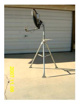
A Radio Shack 3 foot roof mount makes a nice tripod for fieldwork. It has a hole for 1.5-inch pipe or electrical conduit. You can build a platform to hold your electronics package. The TV satellite dish has elevation adjustment. Coaxial conduit allows azimuth rotation. Radio Shack has a 5-foot version of this tripod.
