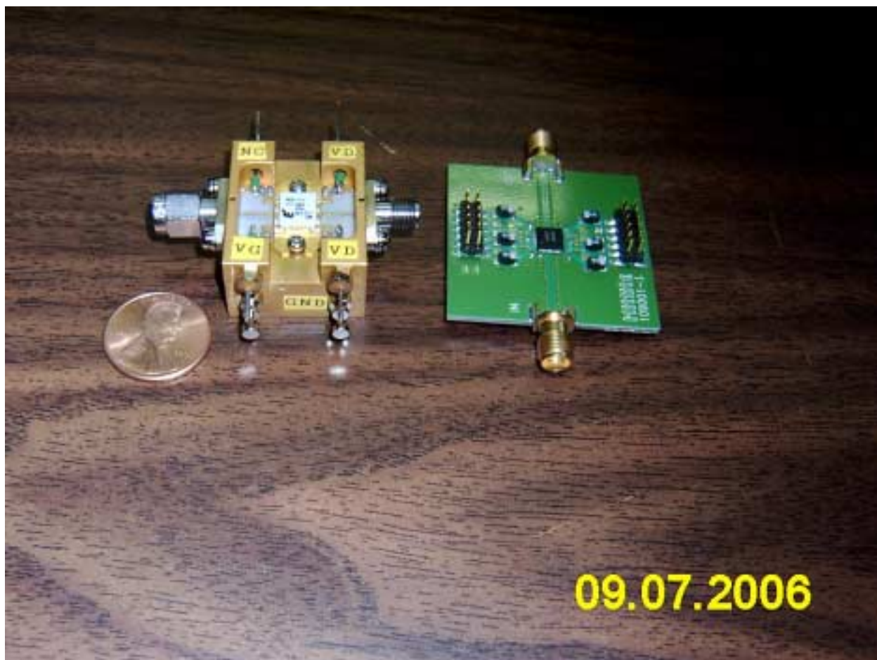
Frank's, WB6CWN Hittite demo board 10 GHz 2w amp and the Eudyna similar device
