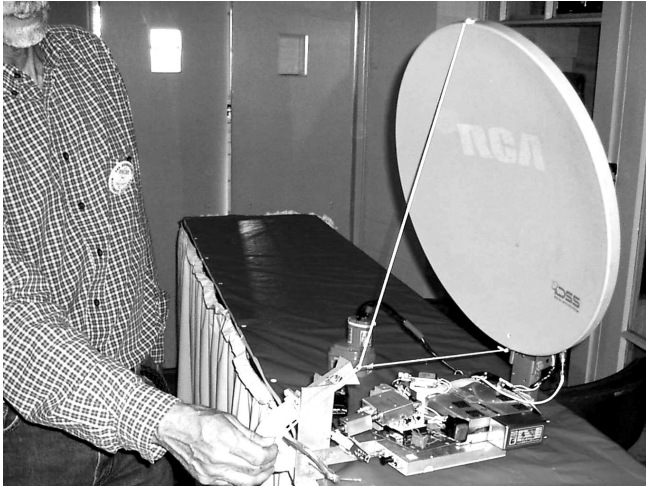
The method described by Paul Wade W1GHZ to locate the proper offset fed dish feed point is used to open the dish to the correct angle.
