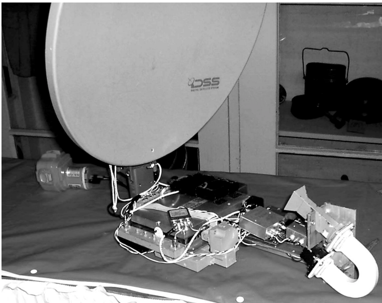
The only waveguide is from the horn to the T/R relay. All the transceiver components are double side taped to the support arm that comes out at a location below the normal feed bracket. This change of bracket and location of hardware keeps the “balance pint” to where it is an easy hand held point and shoot.
