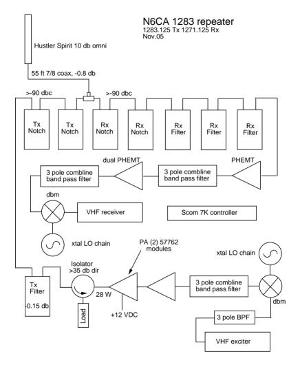
N & SMA connectors used throughout. Male connectors are Silver crimp N with Gold pins, RG142 coax cable Tx filter eliminates out of band sigs beyond directivity BW limit of isolator see: http://www.ham-radio.com/n6ca fo repeater construction details
